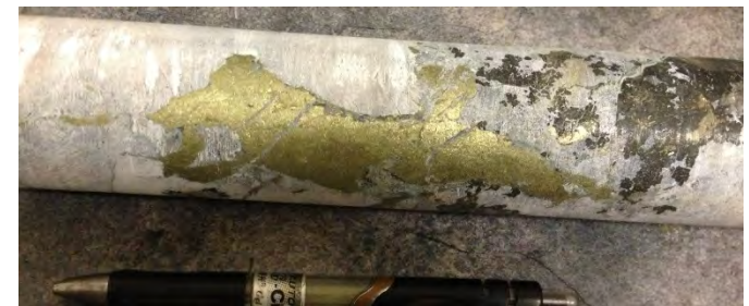
2013 – Diamond drilling – Mount Colin West – chalcopyrite sulphide mineralisation intersected in core. Targeting extensions to the Mount Colin deposit
