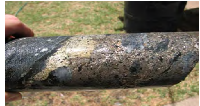
2012 – Diamond drilling – FC4 – chalcopyrite sulphide mineralisation intersected in core. Targeting Ernest Henry style IOCG deposits
