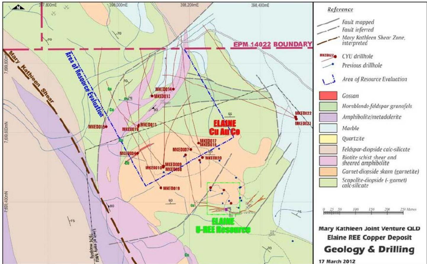
Figure 2. Simplified map showing north side of the Elaine garnet hill. Mineralisation is expected to continue down the western side and on the southern side of the hill and merge with the U-REO Resources where untested copper outcrops occur.
