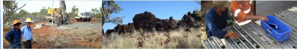
**Xinzhai Drilling** – Hole XZP001 is to test the dipping extension of known mineralisation defined by trenches and adits. Visual copper silver intercepts, assay results due in coming weeks.
