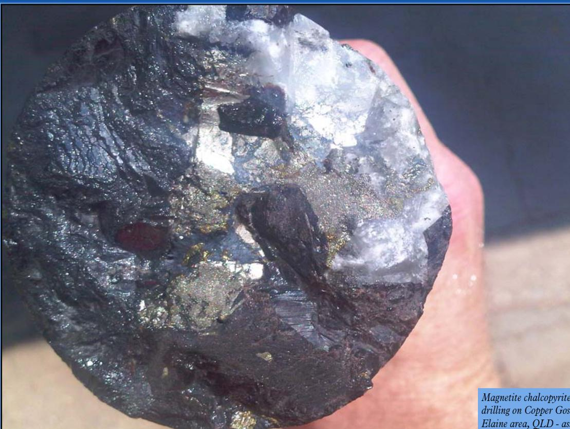
Magnetite chalcopyrite pyrite core from drilling on Copper Gossan prospect, Elaine area, QLD - assays are awaited.
