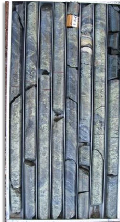
*High grade copper mineralisation from Sandiego Cu-Zn deposit. 8.4m at 10.68%Cu, 0.35%Zn, 1.2g/tAu, 20g/tAg and 0.5%Co from 393.6m - diamond hole SRCD 064*
