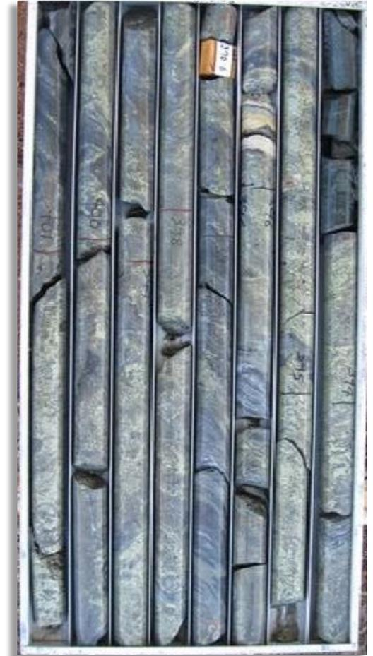
*High grade copper mineralisation from Sandiego Cu-Zn deposit. 8.4m at 10.68%Cu, 0.35%Zn, 1.2g/tAu, 20g/tAg and 0.5%Co from 393.6m - diamond hole SRCD 064*
