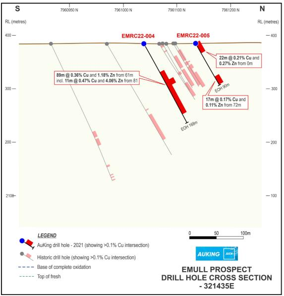
Figure 3. Emull drillhole cross-section plan (holes EMRC22004 and 005)
