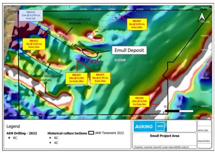
Figure 2. Emull Deposit showing location of drill holes and potential mineralised extensions to the north-west and south-west.
