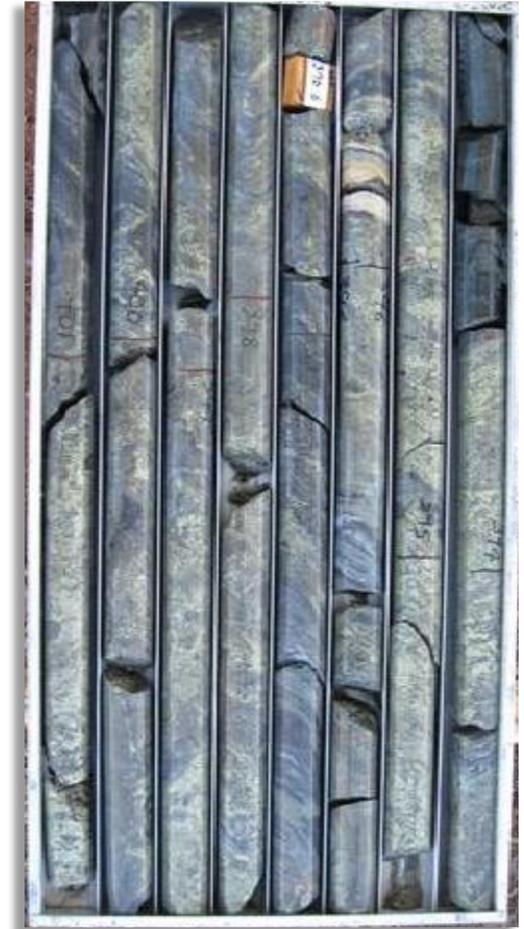
*High grade copper mineralisation from Sandiego diamond hole SRCD064*
