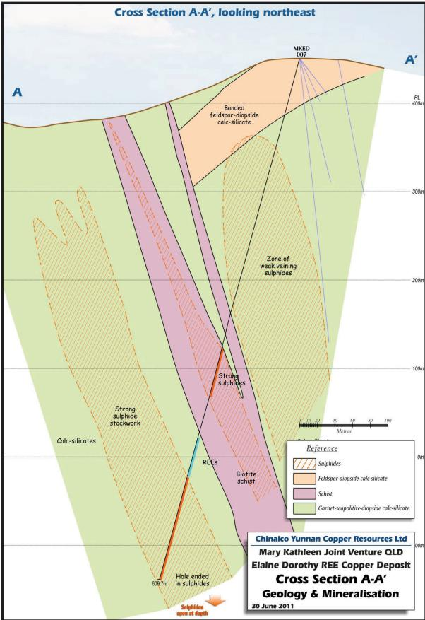
Figure 4.. Cross Section looking NE.
