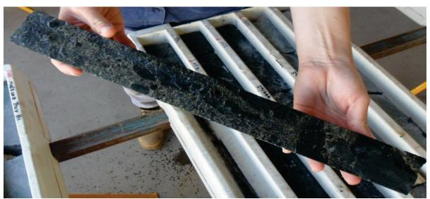
**Plate 3. MKED008.** Disseminated pyrrhotite (iron sulphide) matrix with disseminated chalcopyrite (copper sulphide) 453 metres.
