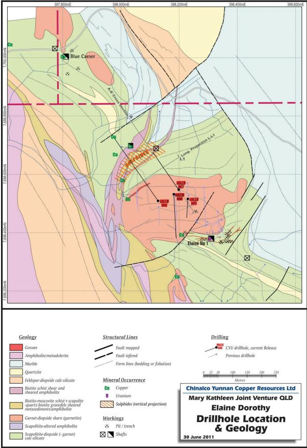
**Figure 2.** Prospect and drillhole location plan for the Elaine prospect of the Mary Kathleen Joint Venture Project with Goldsearch Limited. Further scout drilling is planned to be undertaken on the southern Cerium (Ce – REE) and Copper geochemical anomalies.
