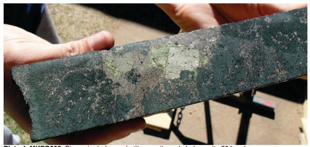
Plate 4. MKED008. Disseminated – pyrrhotite – pyrite and chalcopyrite 504 metres.
