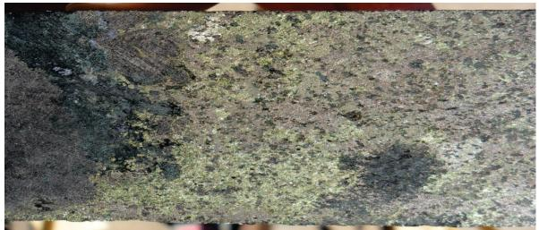
Plate 2. MKED008. Disseminated chalcopyrite - pyrrhotite 423 metres.
