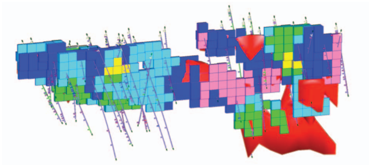
Figure 4: Block model of the Gem resource, looking to the northwest. (Colours: pink <0.1% copper; blue = 0.1-0.2 copper; cyan = 0.2-0.5 copper; green = 0.5-1.0 copper; yellow = 1-2.5% copper. The red areas represent the geological interpreted wireframe for the mineralisation). Note two higher grade copper zones in the north and south, and the possible extension of mineralisation to the south and at depth.
