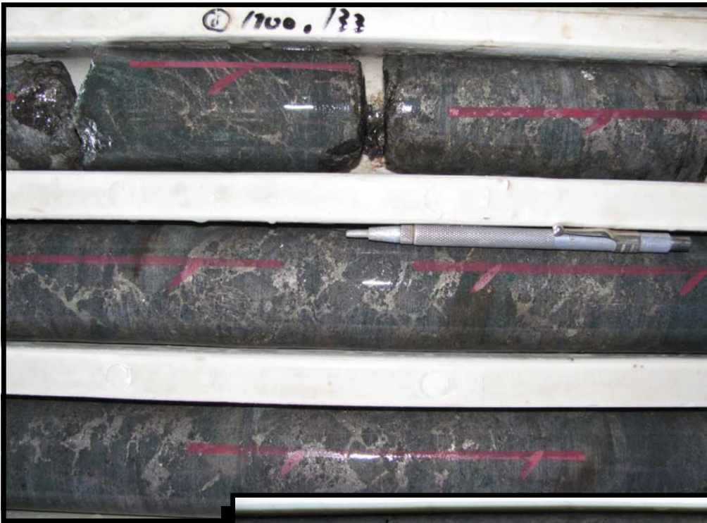
Left. Pyrrhotite-pyrite stringer zone through garnetite skarn (around 48m).
