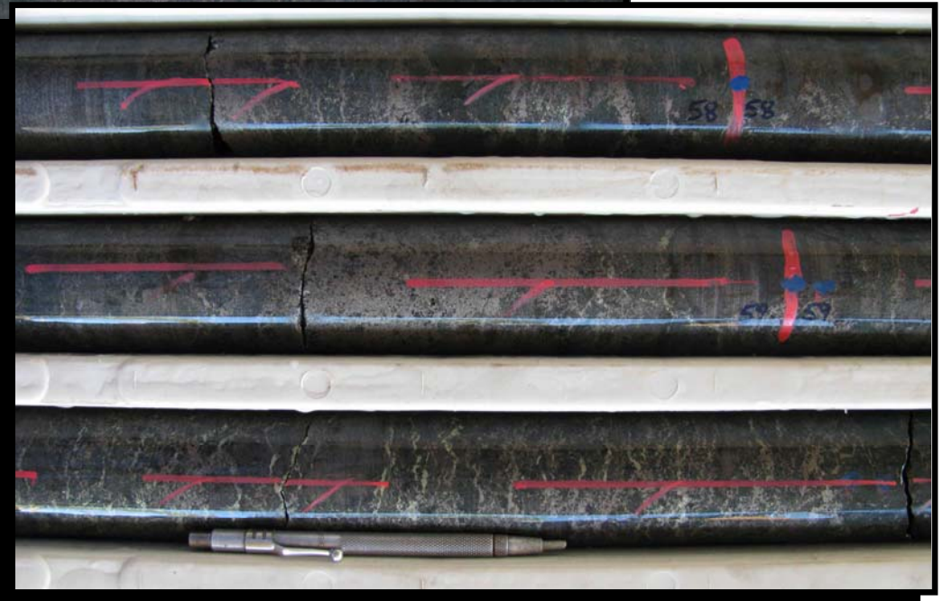
Right. Strong pyrrhotite-chalcopyrite-pyrite zone through garnetite skarn (around 58 – 60m). Below. Close up of strong pyrrhotite-chalcopyrite-pyrite zone through garnetite skarn.
