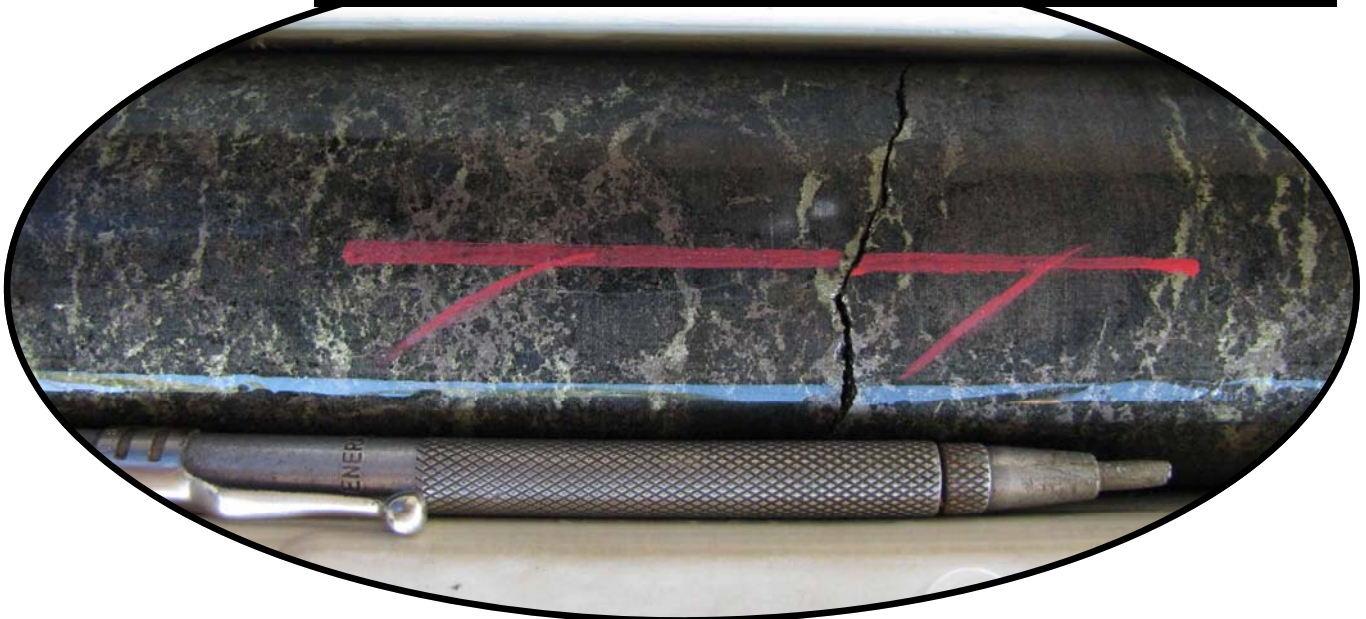
Right. Strong pyrrhotite-chalcopyrite-pyrite zone through garnetite skarn (around 58 – 60m). Below. Close up of strong pyrrhotite-chalcopyrite-pyrite zone through garnetite skarn.
