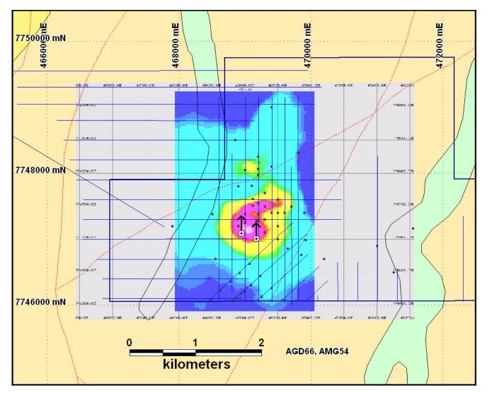
Figure 3. A depth slice at 337m depth of the FC4 target showing an untested IP response. The target exists from 100m to below 400m depth. Proposed drillholes, shown as arrows, are planned to commence in early December.
