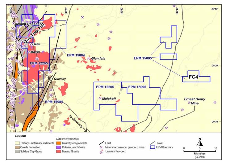
Figure 2. The FC4 Prospect is less than 6 kilometres north of Ernest Henry mine leases. The One Tree Hill prospect is also depicted. CYU is currently undertaking geophysical and geochemical programs over the One Tree Hill prospect.
