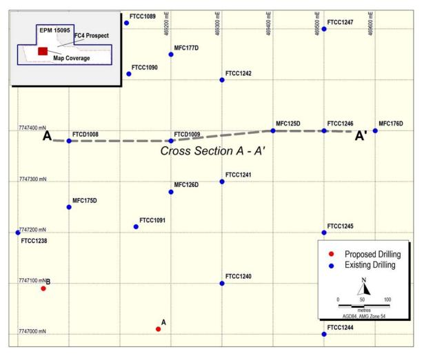
Figure 3. Proposed diamond drill holes are going to be drilled deeper and further south than previous drilling to test an undrilled IP response similar in dimension to Ernest Henry.
