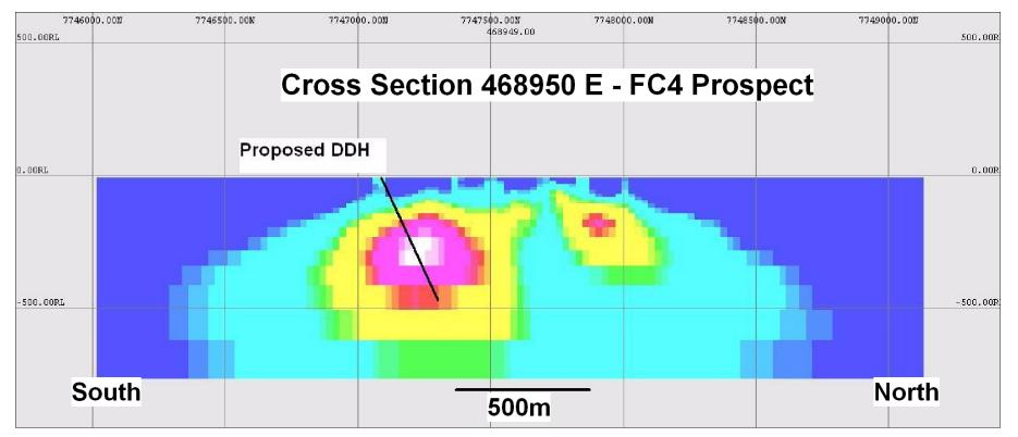
Figure 5. FC4 prospect. Section 468950E showing trace of proposed drill hole.
