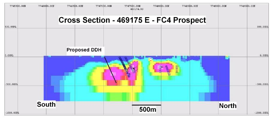
Figure 4. FC4 prospect. Section 469175E showing trace of proposed drill hole.
