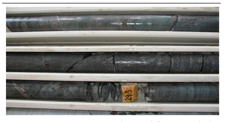
MKED003, 27.8 to 29.4 metres - Strong disseminated allanite-uraninite bands +calcite+pyrite in a diopside calc-silicate. Assayed 1m @ 3.99 kg/t  $U_3O_8$ , 7.56% TREO from 28.5m within a broader zone of 3.5m @ 1.60 kg/t  $U_3O_8$ , 3.81% TREO from 27.50m
