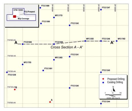
Figure 3. Location of two diamond drill holes which will be drilled deeper and further south than previous drilling to test an undrilled IP response similar in dimension to the Ernest Henry orebody.
