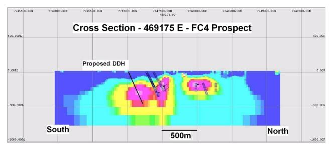
Figure 5. FC4 Prospect. Section 469175E showing trace of drill hole CCDD001.
