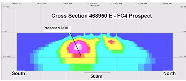
Figure 6. FC4 Prospect. Section 468950E showing trace of drill hole CCDD002.
