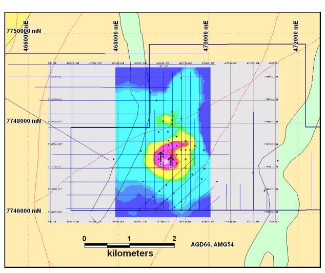
Figure 4. A depth slice at 337m of the FC4 target showing an untested IP response. The target exists from 100m to below 400m depth. The CYU drillholes are shown as arrows.
