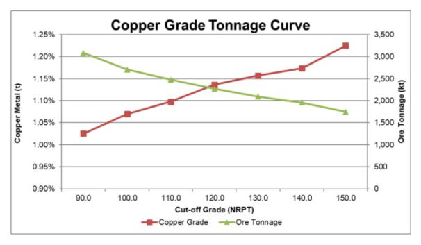
Figure 6-10: Copper Grade Tonnage Curve
