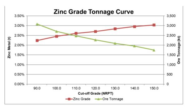
Figure 6-11: Zinc Grade Tonnage Curve
