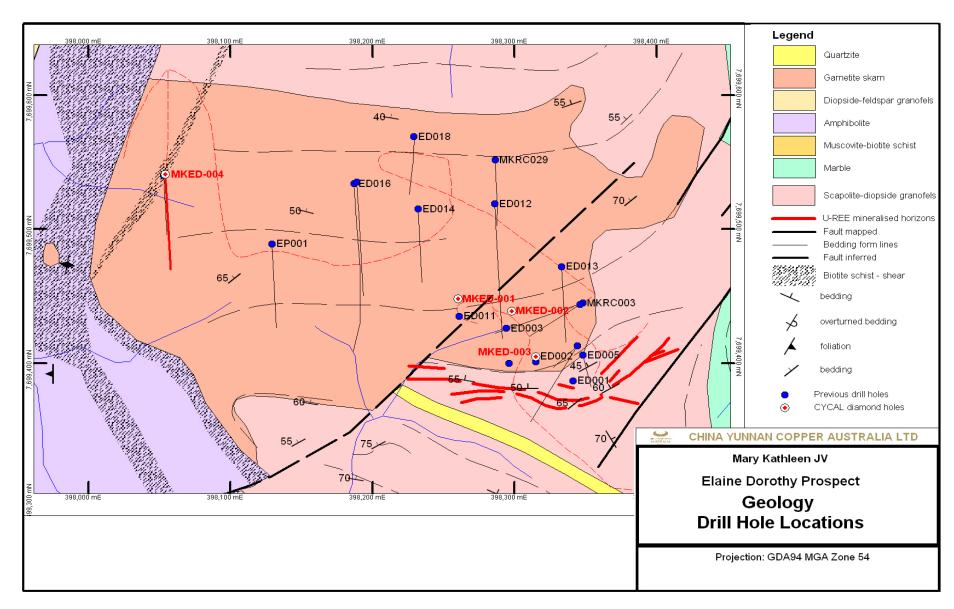
Figure 2. Drillhole Location and Geology Plan
