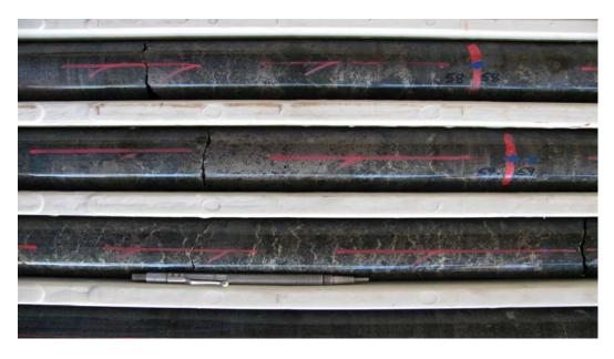
**Photo 1:** MKED004, ~57.00 to 60.00 metres - Strong fracture controlled phyrrhotite+pyrite+chalcopyrite mineralisation in a garnetite and diopside calc-silicate units. Assays returned for **interval = 3m @ 1.04% copper, 361ppm cobalt and 0.09g/t gold**.
