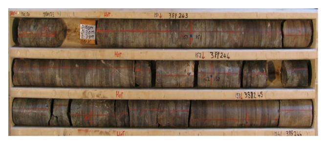
**Photo 2:** MKED004, ~151.00 to 153.00 metres – REE mineralisation associated with carbonate-magnetite-tremolite alteration. Presence of black mineral laths, tentatively identified as allanite Assays returned for interval = 2m @ 4427ppm TREO and 0.15 kg/t  $U_3O_8$
