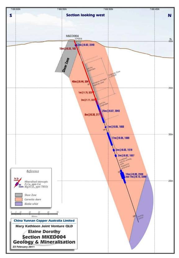
**Figure 3.** Section 398050mE – MKED004 & EP004. Red intercept depicts copper cobalt zone and blue is REE Uranium Zone. This polymetallic intercept is open to the north and south and will represent resource growth for REE and a new copper cobalt zone for further delineation.
