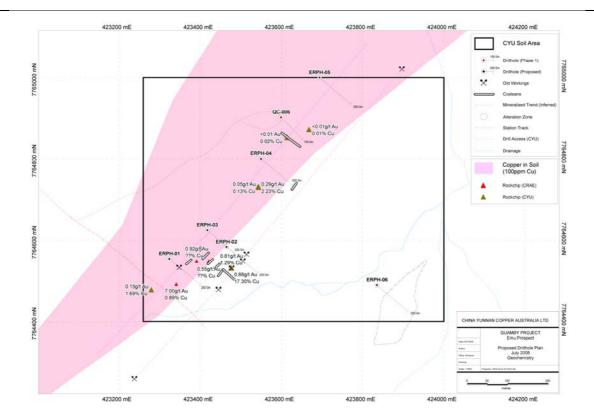
**Figure 3** Interpretation of mineralised zone for Emu Prospect. Sampling of nearby trenches has resulted in strong anomalies which combined with IP results indicate robust drill targets for the forthcoming quarter.
